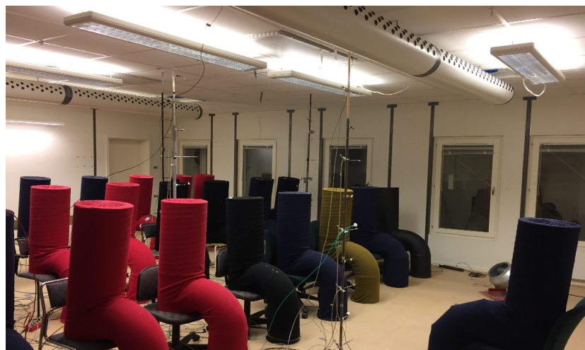
Figure 2. Set-up of measurement points and mannequins. (Top) Measurement points and placements of SJ and confluent jet devices, red mannequins were turned on for the 10 p (persons) cases, red and blue were turned on for 19 p cases and red, blue and yellow were turned on for the 28 p cases. (Bottom) Photo of set-up.
